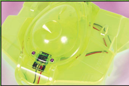
FIGURE 19. Snap the IR sensor holder into the hinge along the front of Binary Player Robot.
